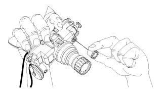
Figure 2-12. IR Spot/Flood Lens Installation.
